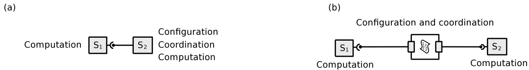
Figure 5: Organizing dependencies between services. (a) The traditional approach where services depend directly on each other. (b) Our approach: independent services are composed using a separate mechanism.
